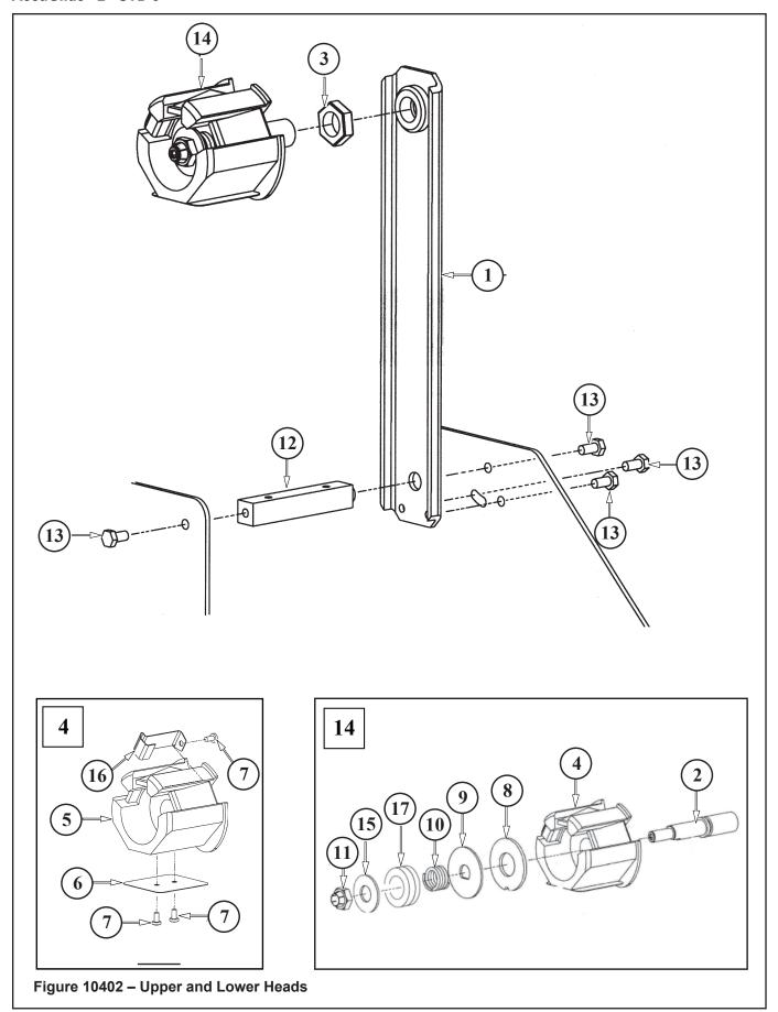
Figure 10402 – 3" Latch Upper and Lower Heads
