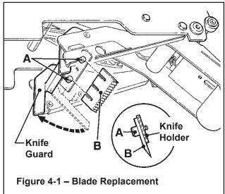
3. Bottom the blade slots against the screws. (This will position the blade at the correct angle.)
