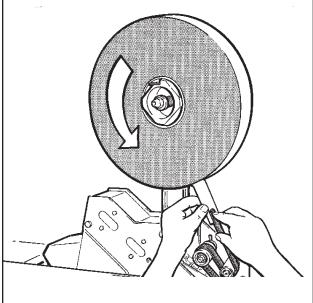
Figure 3-4 - Tape Loading/Threading
