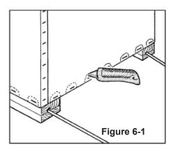
After cutting out or removing the staples, lift the shipping box in order to clear the machine *Note:* Two (2) persons required.
