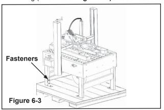
Remove the leg height adjustment cap screws and replace with the cap screws from the tool kit. Loosen both cap screws. Remove and replace them one at a time to keep the inner threaded plate in position.
