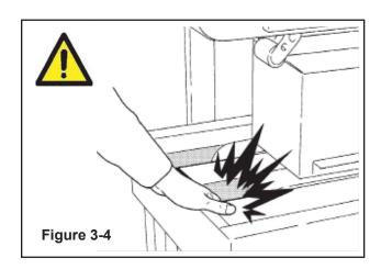
*Important* - Cavity in the conveyor bed. Never put your hands inside any part of the machine while it is working. Serious injury may occur (Figure 3-4).
