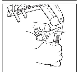
Figure 3-5 - Tape Loading/Threading
