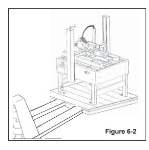
Transport the machine with a fork-lift truck to the operating position.
