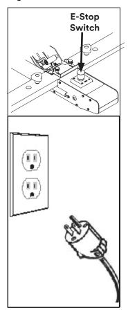
The machine is provided with a LATCHING EMERGENCY STOP BUTTON (Figure 3-1); when this button is pressed, it stops the machine at any point in the working cycle. Maintain clear access to power cord while machine is operating. Disconnect plug from power source before machine maintenance (Figure 3-1).
