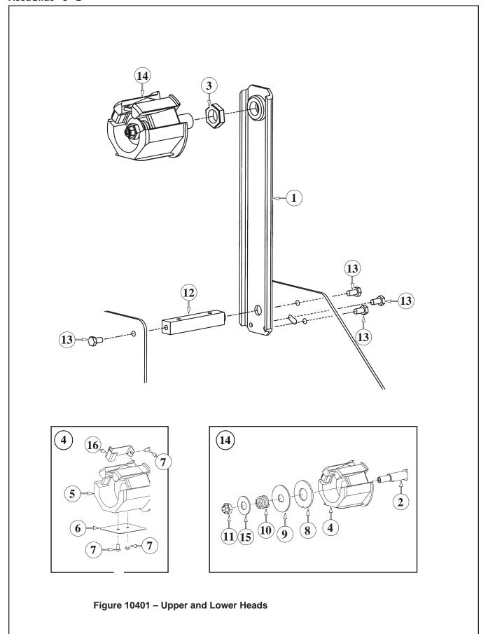
Figure 10401 – 2" Latch Upper and Lower Heads
