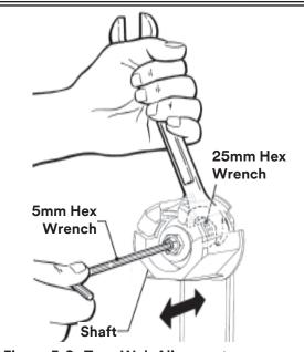
Figure 5-2 Tape Web Alignment
