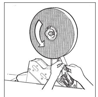
Figure 3-4 Tape Loading/Threading
