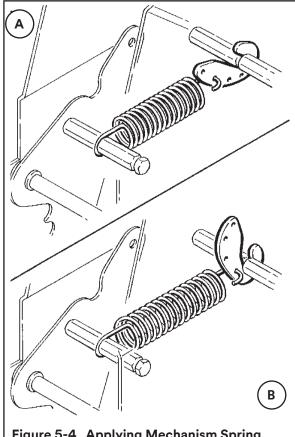
Figure 5-4 Applying Mechanism Spring
