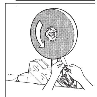
Figure 3-4 Tape Loading/Threading
