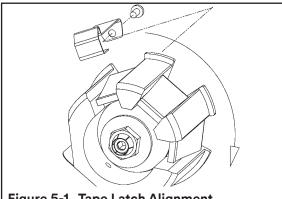
Figure 5-1 Tape Latch Alignment
