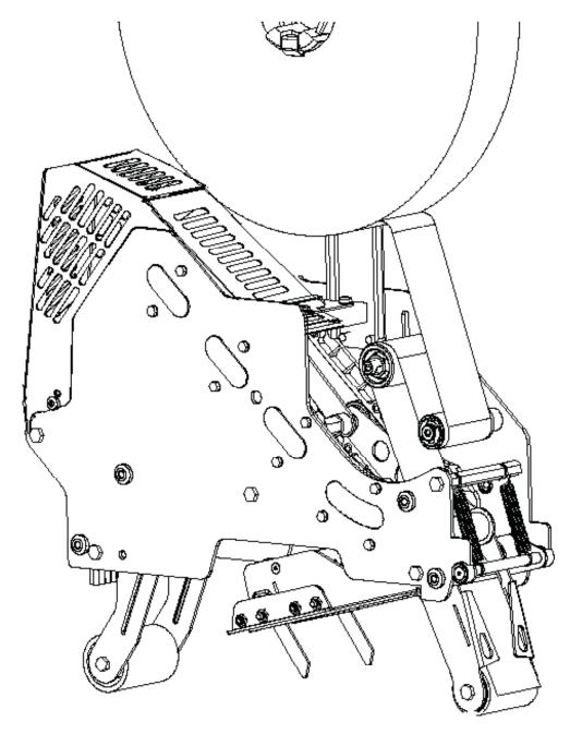
AccuGlide™ 3 Upper Taping Head - 2 inch, Type 11400
