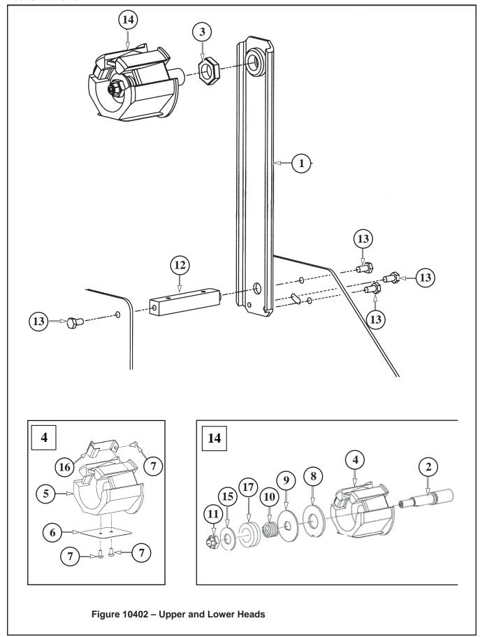
Figure 10402 – 3" Latch Upper and Lower Heads
