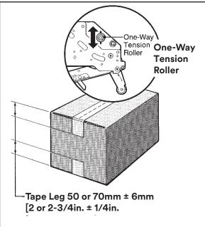
Figure 5-6 Leading Tape Leg Length
