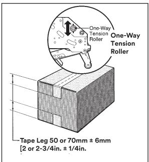
Figure 5-6 Leading Tape Leg Length
