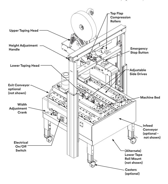
Figure 3-9 8000a-8000a3 Case Sealer Components (Left Front View)
