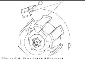
Figure 5-1 Tape Latch Alignment
